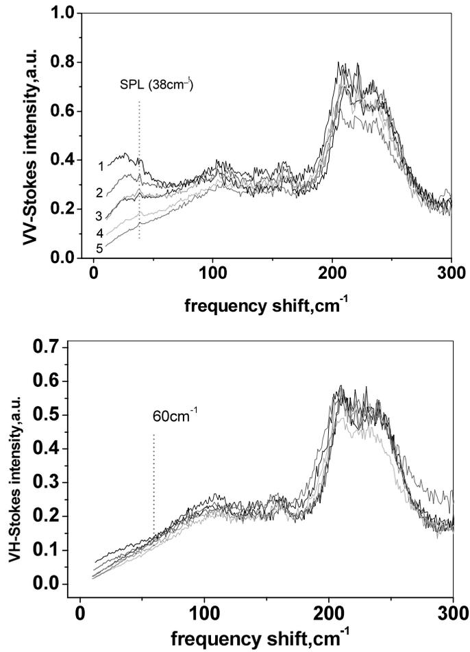
**Figure 6.** Low-frequency RS for sample 4 (normalized VV and VH Stokes spectra, reduced by factor  $f$ ); 1: 30; 2: 50; 3: 100; 4: 150; 5: 200 K. SPL—source plasma line (elastic scattering of the laser 488.9033 nm light).
