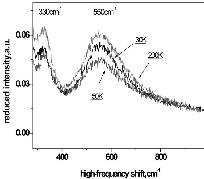
**Figure 3.** The high-frequency Stokes Raman spectra for NaCl:KBF<sub>4</sub> (sample 4, with 5.7 mol% Na) measured at 30, 50, and 200 K.
